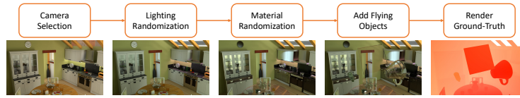
Fig. 5: Synthetic dataset generation pipeline. We perform these steps to boost the frequency of non-Lambertian object appearances and the diversity of rendered images.
